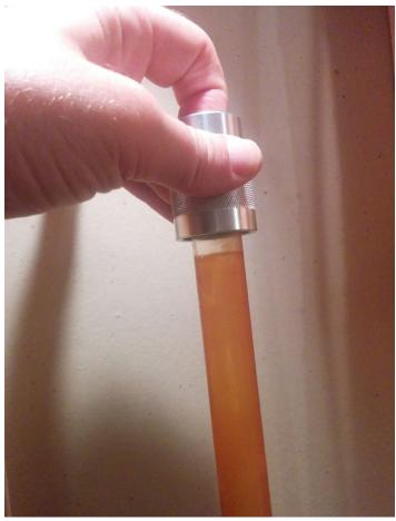
Make sure that the ultraviolet light bulb sleeve is cleaned on a regular basis. If the sleeve is dirty, the ultraviolet rays cannot properly inactivate the germs in the water, allowing contaminated water to flow through untreated.
