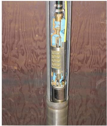
A submersible pump in a drilled well casing model.
